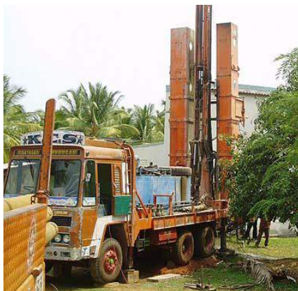
Fig 5.3: A borewell rig, mounted on a lorry, for deepening or digging borewells
